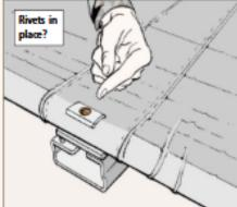
If the hinge on the spreader bar sticks or shows signs of corrosion, give it a shot of WD-40 or a similar lubricant. That'll loosen rusted parts and protect the metal against moisture. NSN 8030-01-418-9008 gets you an 11-oz aerosol can.
